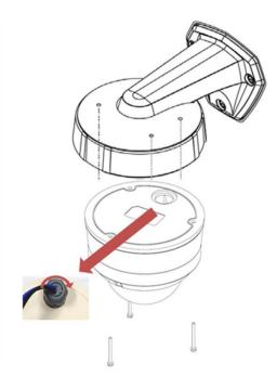
1. Assemble the wall mount bracket assembly..
