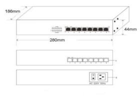
A. Gigabit PoE Port B. AC 220V/50Hz Input
